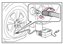
8 Make sure that the compressor switch is off.
