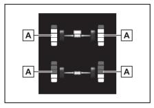
A Torque distribution display Displays the drive status of each wheel in 6 steps from 0 to 5.
