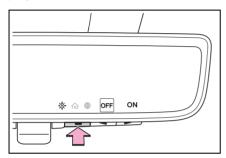
3 Press or to enable (ON)/disable (OFF) the automatic anti-glare function.
