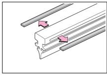
Insert the wiper insert starting from the claw at the center of the wiper blade. Pass the wiper insert through the 3 claws so that it sticks out from the stopper, and then pass the wiper insert through the final remaining claw.
