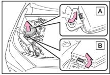
Engine compartment: Type B fuse box
