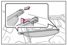
2 Pull out the luggage cover and hook it onto the anchors.
