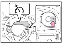
Accelerate or decelerate, with accelerator pedal operation, to the desired vehicle speed (at or above approximately 20 mph [30 km/h]) and press the "-SET" switch to set the speed.
