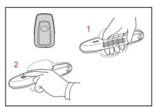
1 Grip the driver's door handle to unlock the door. Holding the driver's door handle for approximately 2 seconds unlocks all the doors. Grip the front passenger's door handle or rear door handle (some models) to unlock all the doors\*.
