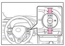
Increases the speed (Except when the vehicle has been stopped by system control in vehicle-to-vehicle distance control mode)
