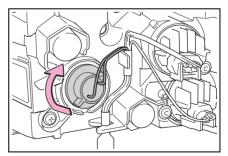
6 Align the grooves on the light unit with the claws, and insert the light unit straight so that the pin on the light unit fit into the hole. Confirm that the light unit is completely secured.
