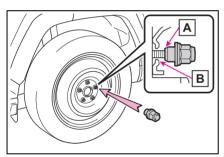
When replacing an aluminum wheel with an aluminum wheel, turn the wheel nuts until the washers ( $\boxed{\mathbf{A}}$ ) come into contact with the disc wheel ( $\boxed{\mathbf{B}}$ ).
