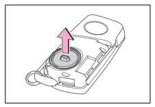
3 Remove the depleted battery.
