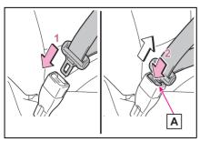
To fasten the seat belt, push the plate into the buckle until
